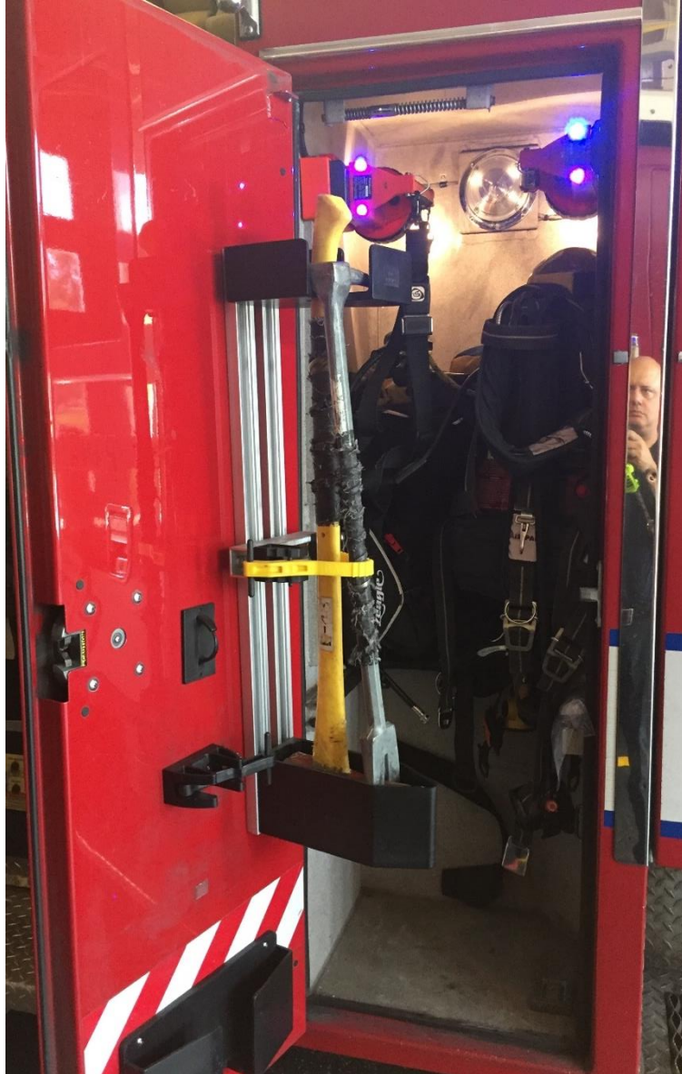
Relocation of SCBA and tools to outside compartments (Pierce Dash – 2007) Picture 1
