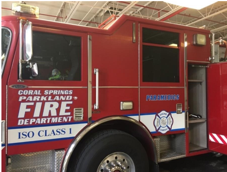
Relocation of SCBA and tools to outside compartments (Pierce Dash – 2007) Picture 2
