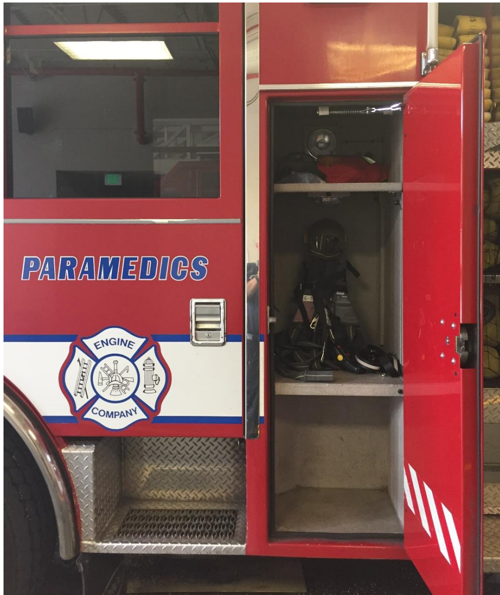
Relocation of SCBA and tools to outside compartments (Pierce Dash – 2007) Picture 3
