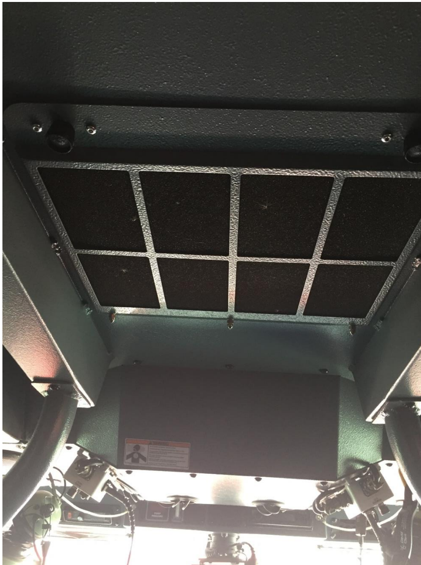
New Clean Cab AC filter with knobs to easily open and clean filter.
